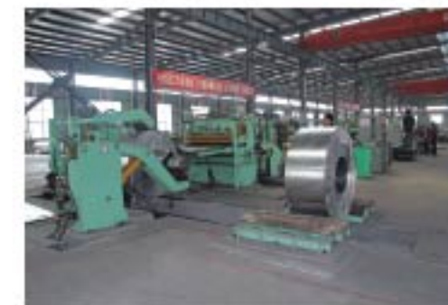
1. Steel Roll Cutting
